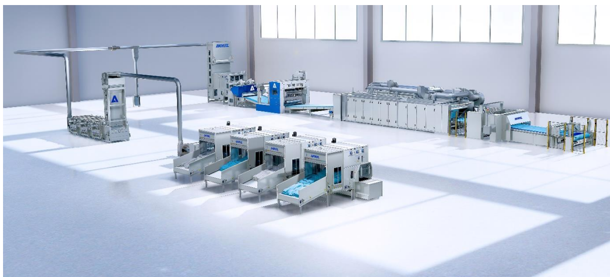
neXline airway for the production of durable nonwovens dedicated to automotive, building insulation and mattress end-uses
